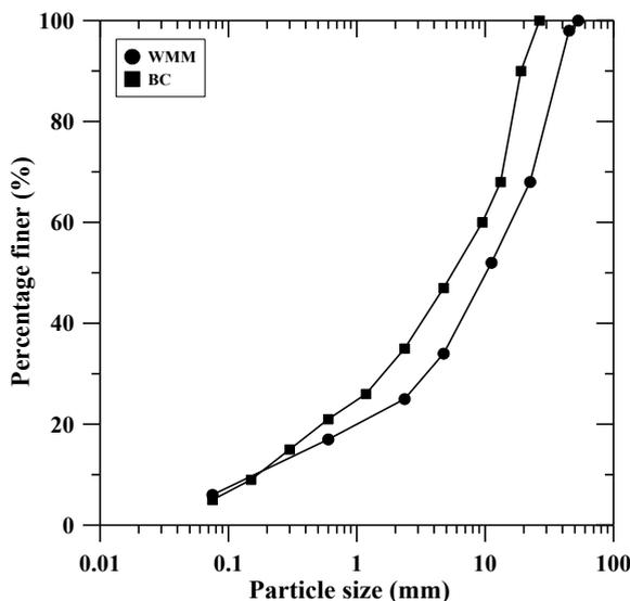
**Fig. 1** : Particle size distribution curve for WMM and BC materials
