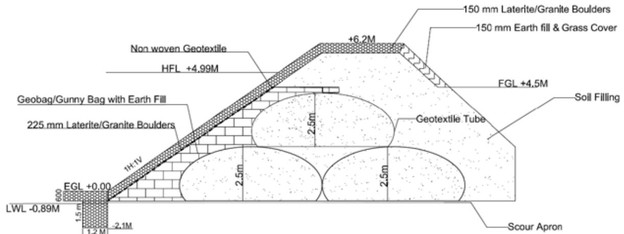
Fig. 3 : Cross-section of the geotextile tube dyke
