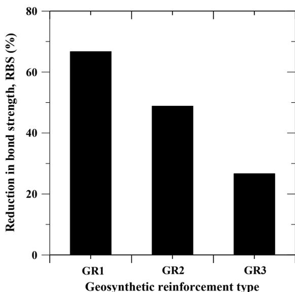
Fig. 8 : Variation of RBS (peak state) with geosynthetic reinforcement type
