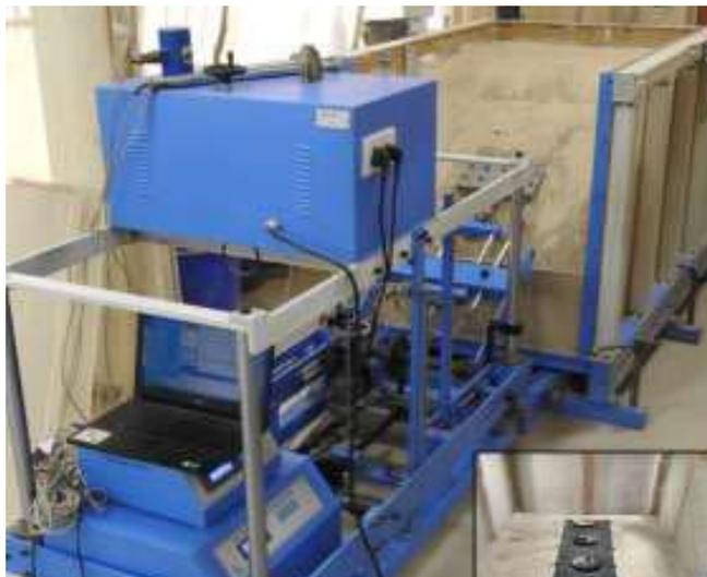
**Fig. 2 :** Inclined pullout test device.
