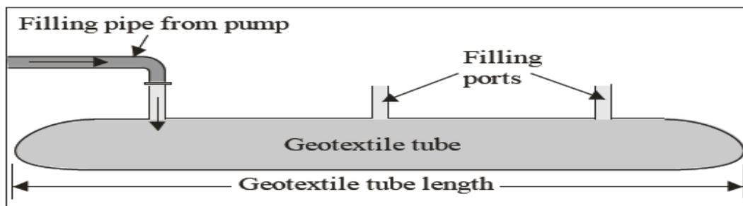
Fig. 4 : Typical features of geotextile tube.
