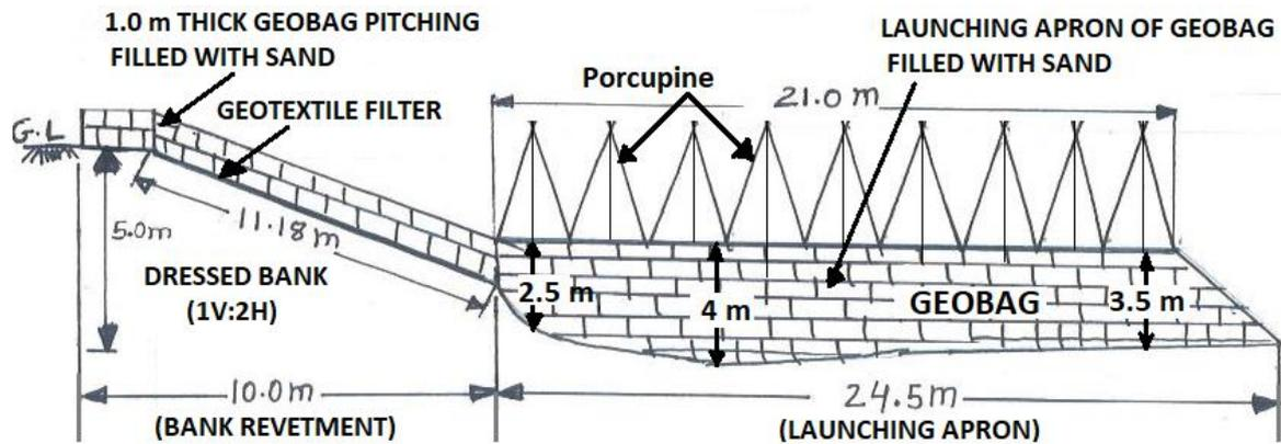
Fig. 10 : Cross section at B-B of transverse protection structure having porcupine spur 21 m length
