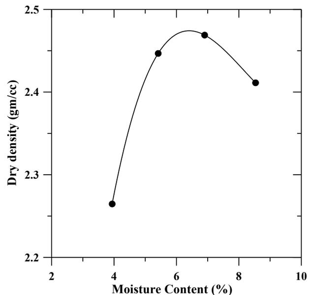
**Fig. 2** : Compaction characteristics of WMM material
