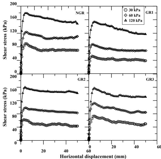
**Fig. 5 :** Variation of shear stress with horizontal displacement for different normal stress applied
