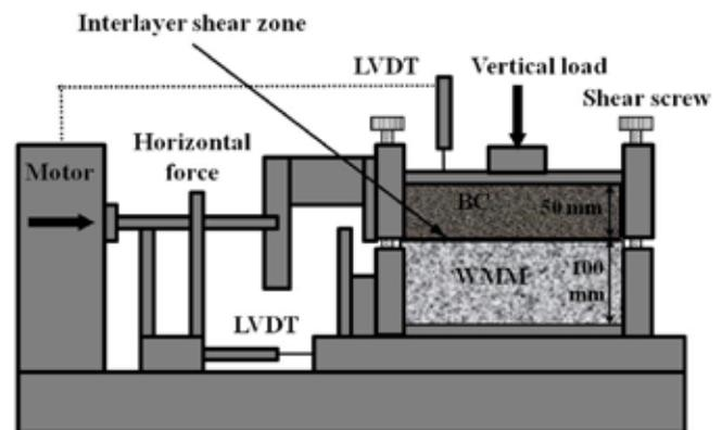
Fig. 4 : Schematic of Interface shear strength test setup
