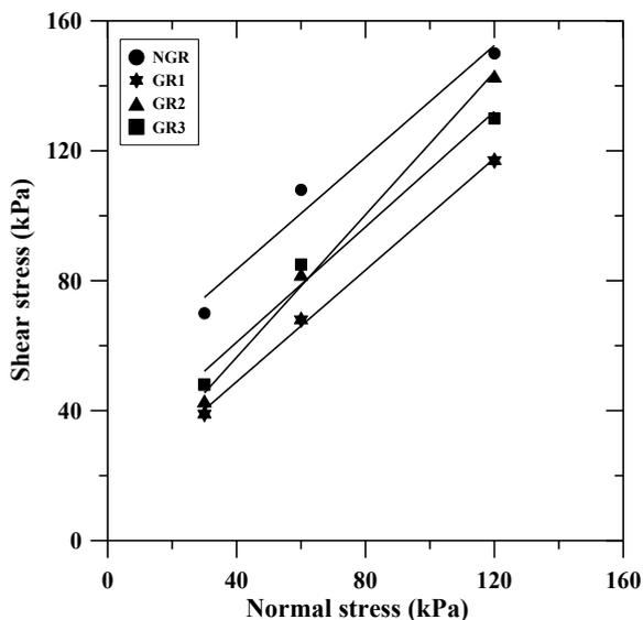
Fig. 7 : Residual interface shear strength characteristics of unreinforced and geosynthetic reinforced pavement layers
