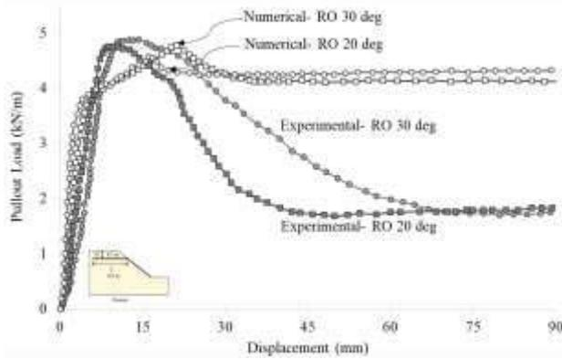
**Fig. 5(b)** : Run-out anchor under inclined pull: Comparison among experimental and numerical plots
