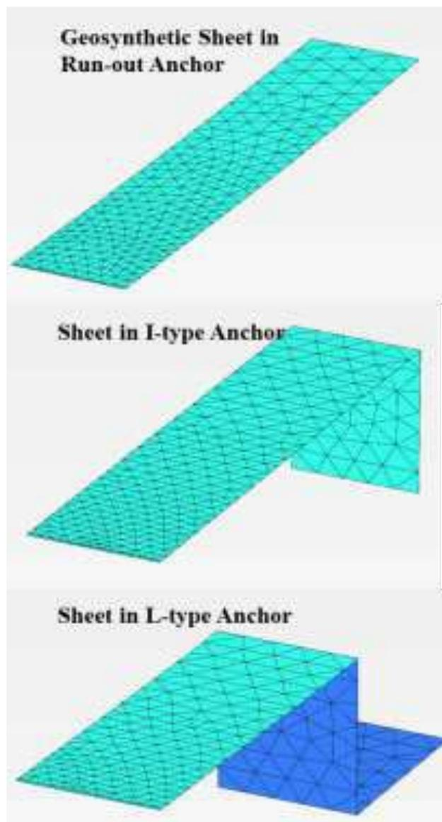
Fig. 4 : FE model of three anchors
