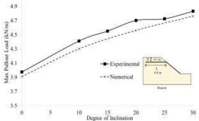
**Fig. 6** : Run-out anchor under horizontal pull: Variation in maximum pullout load with increase in pull inclination
