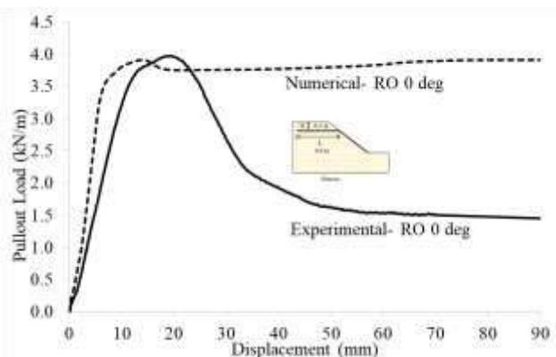
Fig. 5(a) : Run-out anchor under horizontal pull: comparison among experimental and numerical plots
