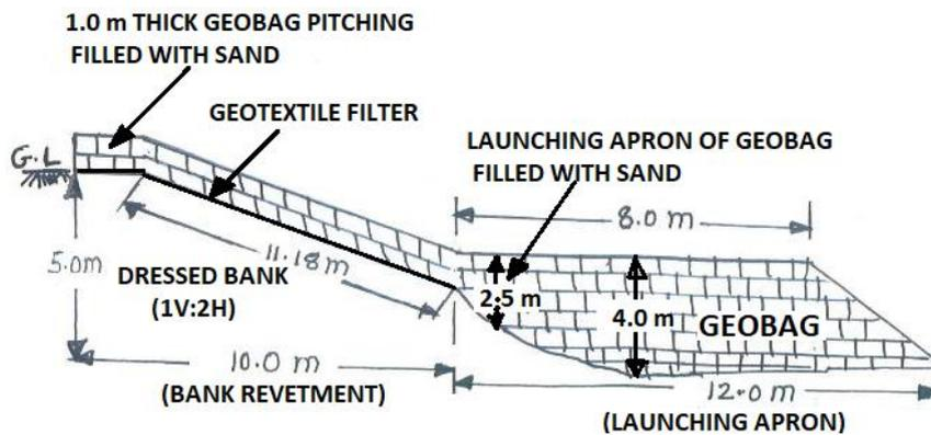
Fig. 9 : Cross section at A-A of longitudinal protection structure
