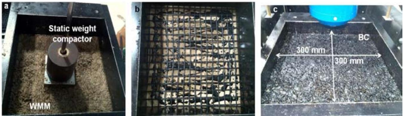
Fig. 3 : (a) WMM material compacted as a base course layer; (b) Geosynthetic reinforcement placed at the interface zone; (c) HMA compacted as a surface course layer
