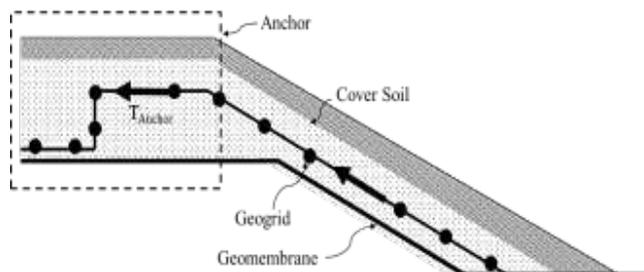
Fig. 1 : Anchorage of veneer reinforcement.
