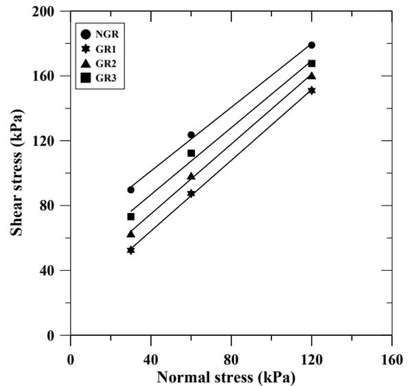
**Fig. 6 :** Peak interface shear strength characteristics of unreinforced and geosynthetic reinforced pavement layers
