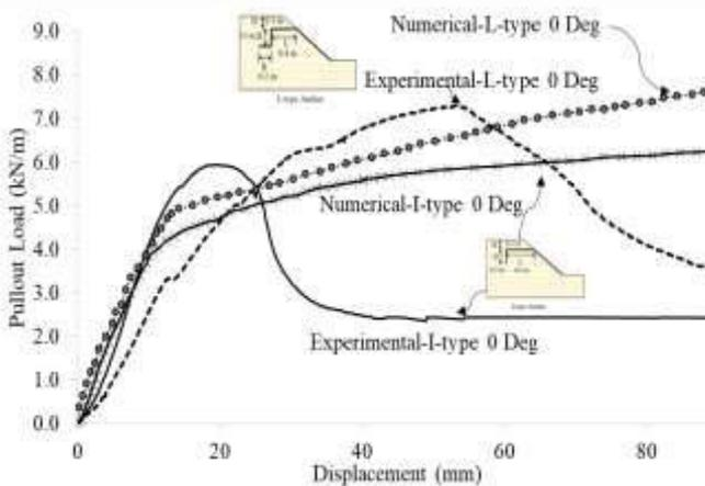
**Fig. 5(c)** : I- and L-type anchors under horizontal pull: Comparison among experimental and numerical plots
